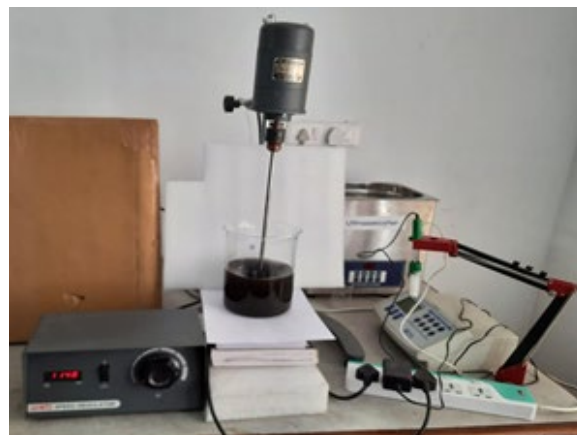
Figure 1: Fe 3 O 4 -Yield stress gel preparation
