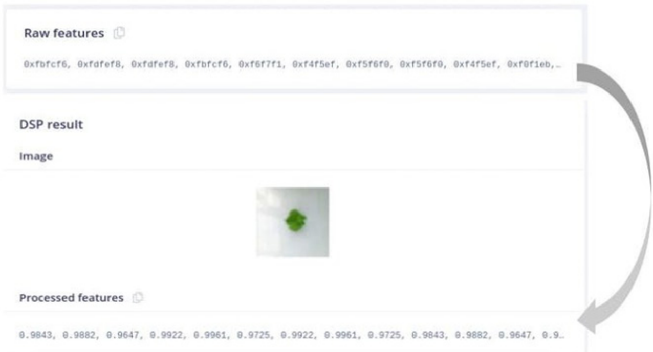
Figure 15: Processing Raw features as processed features
