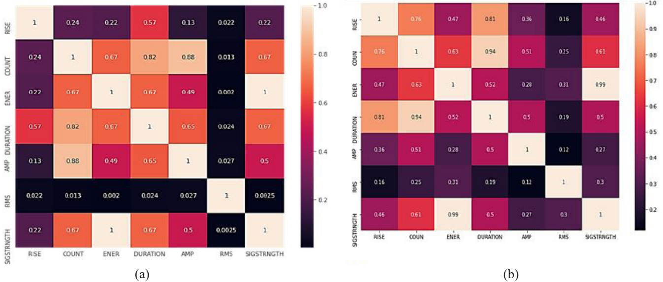
Figure 8: The correlation between AE parameters: (a) 45% of UTS (b) 60% of UTS
