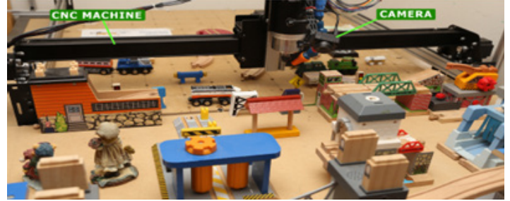
Figure 8: Experimental arrangement viewing a camera straddled on a CNC machine permitting us to capture real information.
