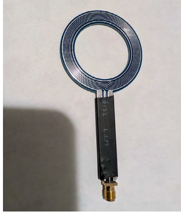
Figure 3: Coil Probe for Measuring Alternating Magnetic Fields
