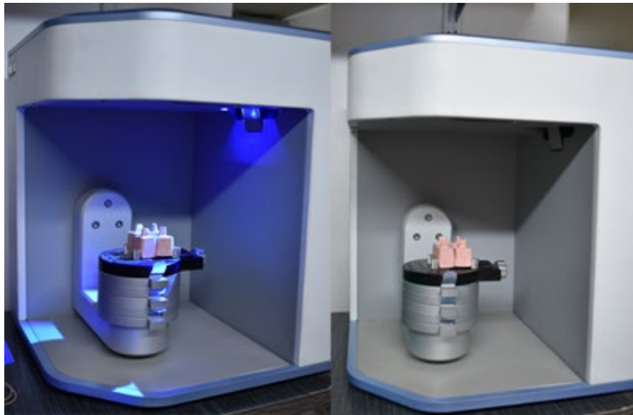
Figure 3: Scanning Casts Using Extraoral Scanner
