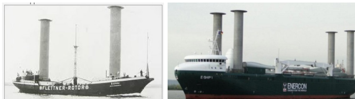
Figure 4: Boats fitted with cylinders rotating to create a forward depression under the effect of the side wind [6,7].
