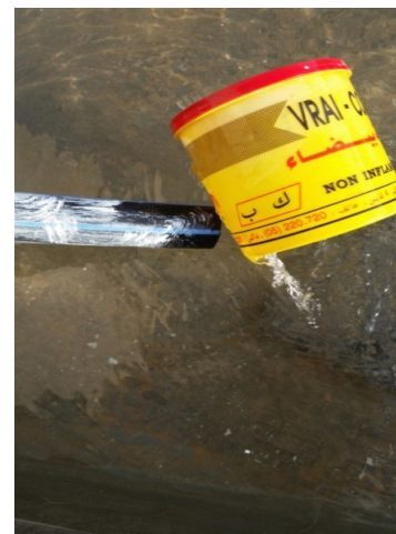
Figure 7: Attraction and rotation of a floating cylindrical object on water by a water jet. Photo Ben Slama R. 2018
