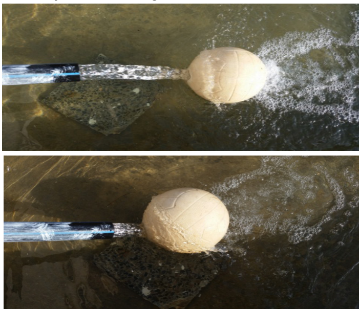
Figure 8: Attraction and rotation of a floating spherical object on water by a water jet. Photo Ben Slama R. 2018
