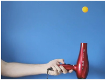
Figure 2: Deviation of an air jet by a rounded obstacle [4].
