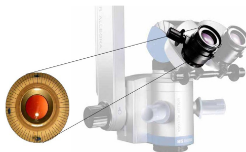
Figure 5: It presents an eyepiece with a scale, mounted to a microscope, facilitating the determination of the axis in the cornea. It is helpful, among others, in the case of toric lens implantation and determining the ranges of limbal relaxing incisions.
