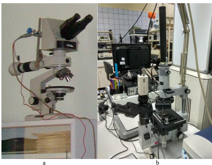
Figure 6: Contemporary Russian Compact Microbeam Setups for Field and (Auto-)Mobile Lab Conditions: a) Combined Laser Diode / DPSSL Compact Microscope for Hydrobiochemical / Geobiochemical and Hydrobiological Microbeam Investigations (GEOKHI RAS, Oleg Gradov, 2010); b) HeNe Laser Microbeam Setup based on Inverted Phase-Contrast Microscope (INEPCP RAS, Andrew Skrynnik, 2017).
