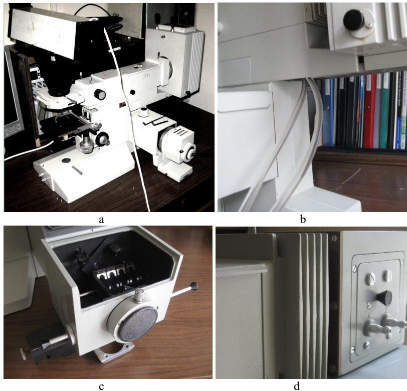
Figure 7: Computerized Multi-Module Multi-Wavelength UV Microbeam Setup with Two Possible Cooling Pathways (O.V. Gradov, Research Center of Neurology, Brain Research Department, Laboratory of Neural Brain Structure, Moscow, 2012-2013).
