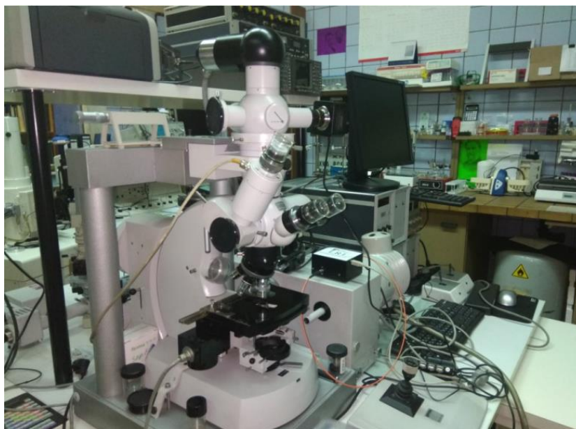
Figure 4: Contemporary Computerized Version of the UV Microbeam Setup based on ZEISS OPTON Photomicroscope with Optical Waveguide Spectrometer, UV Microspectrometer, ZEISS OPTON Micromanipulator and Computer-Assisted Data Acquisition System. Semenov Institute of Chemical Physics, Gradov's Multiparametric Microscopy Infrastructure, 2018.
