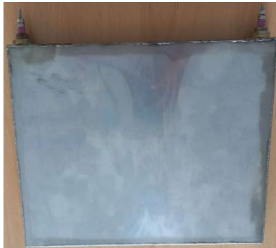
Figure 6: Stainless steel rectangular plate (300 mMX200 mMX20 mM) filled with our materials
