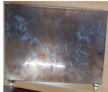
Figure 7: Stainless steel rectangular plate (300 mMX200 mMX20 mM) filled with our materials
