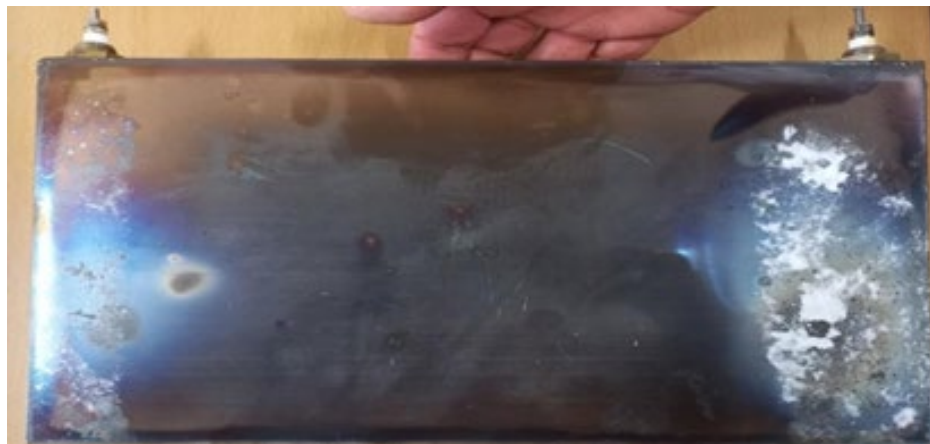
Figure 8: Stainless steel rectangular plate (300 mMX200 mMX20 mM) filled with our materials
