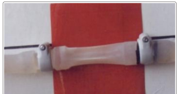
Figure 5: The negative CP (Figure 4) collapses a membrane around the G tube. This means that the G tube irrigates C chamber well under negative pressure without accumulation of fluid. In the case of capillaries shown on the physiological investigation on the hind limb of sheep (see text) arterial flow irrigates ISF space and cells well under negative pressure without oedema formation. While venous flow induces oedema irrespective whether saline or plasma proteins were used. (Reproduced with permission of the author from BHC open access journal; reference 12)
