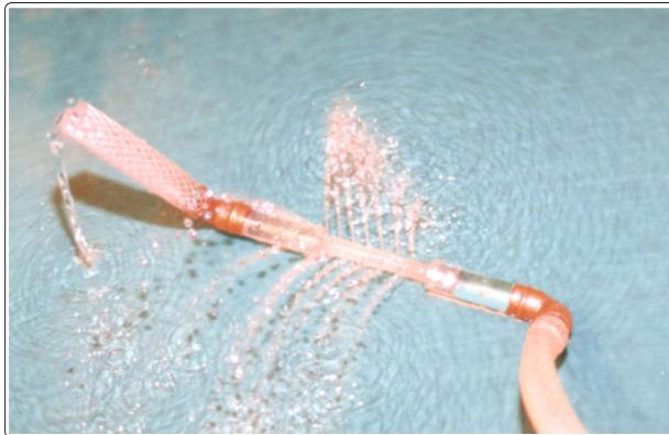
Figure 2: Fluid flows out autonomously through distally situated side holes of a porous orifice (G) tube where SP is positive. Air suction occurs through side holes of the proximal part, as shown in Figure 1, but is not seen here. The fluid around the G tube has magnetic field shape shown above the G tube. (Reproduced with permission of the author from BHC open access journal; reference 12)
