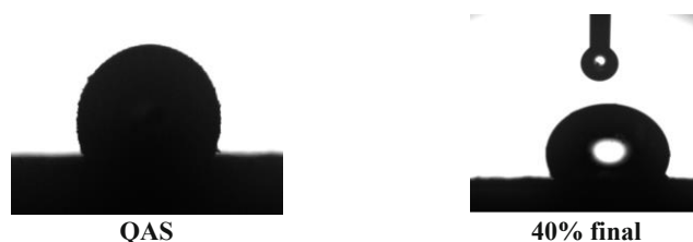
Figure 29 Schematic diagram of contact angle for QAS treated and 40% treated soil.
