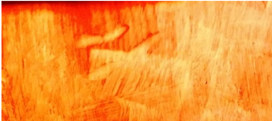
Figure 8: Diffraction lines - Pt sample, horizontal plane, in the center of the photo is an image of fragments of wiring and platinum wire inside the case (SGK) under 7-8 layers of insulating tape
