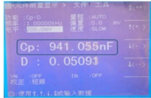
The capacitance was measured at 0.94uF within the spec for C11
