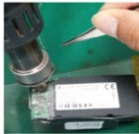
Remove the C11 by heater
