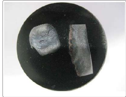
Figure 4: Sample embedded in resin, prepared metallographically and attacked with Nital at 4%
