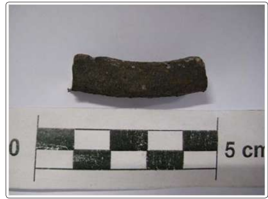
Figure 3: Sample cut from one of the links in the Laredo chain
