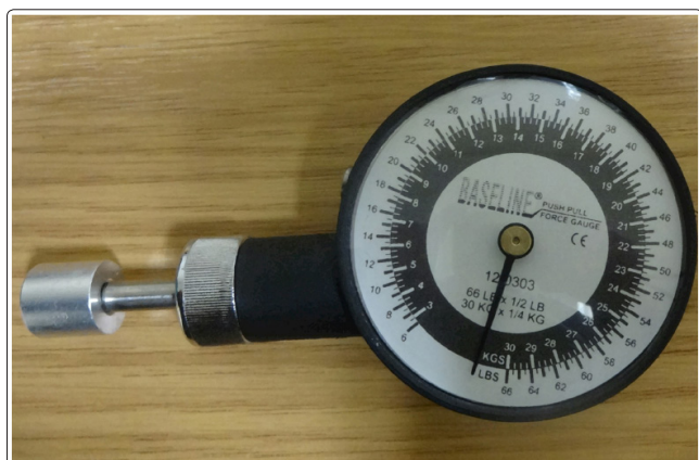
Figure 2: Baseline Dolorimeter (Algometer) with a circular probe
