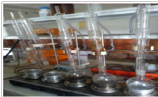
Figure 2.0: Soxhlet extraction of SCG oil
