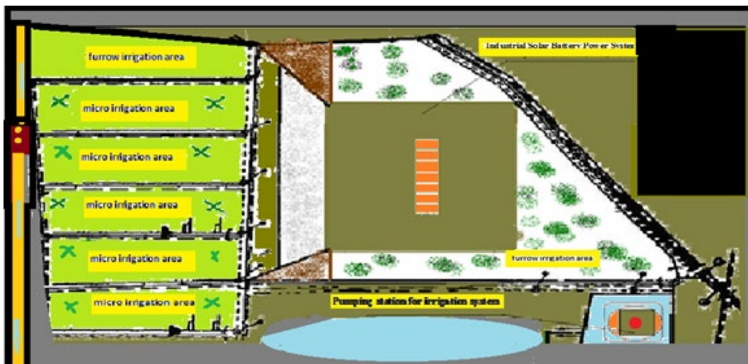
Figure 2: Scheme of the Irrigation Sprinkling Station on the Experimental Part of the Terter RACS in the Garabagh land in the Period 2006-2010 with the use of the Idad and MDR sprinklers
