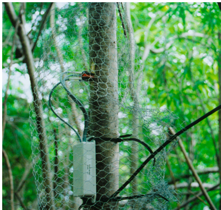
Figure 1: Sap flow sensor and microprocessor attached to stem of Captain Cook tree.
