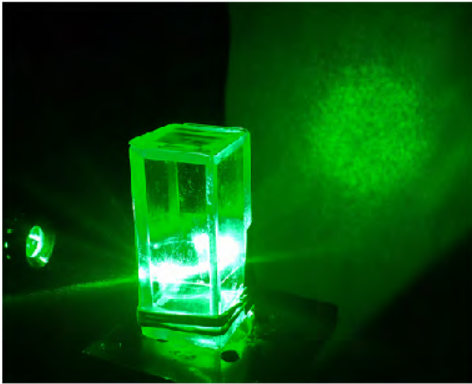
Figure 2: The output laser radiation from the rib of the film on the screen at a distance of 25 cm from the output end.
