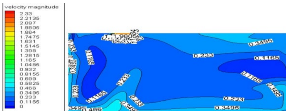
(f) size of indoor unit is 0.5m×0.3m×0.5m
