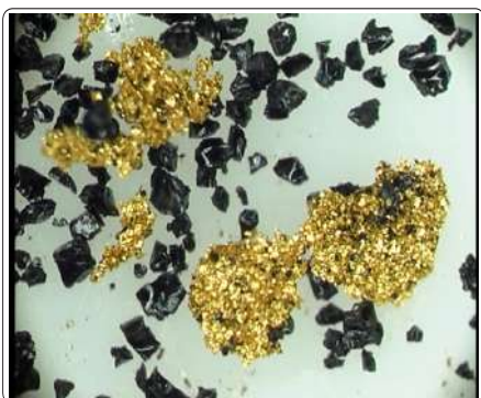
Figure 7: Image of aggregates elemental gold formed in the adsorption on CMA gel observed by optical microscope.
