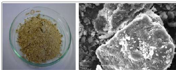
Figure 1: Photograph of residual waste of microalgae, Coccomyxa sp. (left) and its SEM image at magnification of \times 1000 (right).
