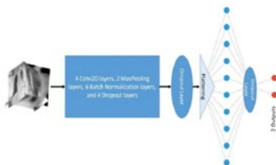
Figure 4: Architecture of CNN with 4 Convolutional Layers
