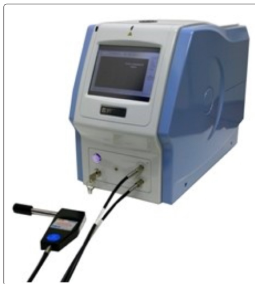
Figure 1: Portable Raman spectrometer with its probe for in-situ analyses
