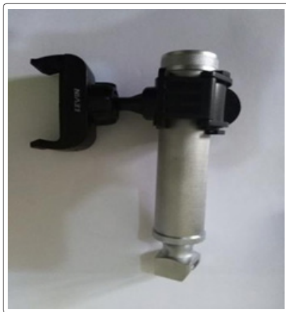
Figure 3: Bike handlebar base adapted to attach smartphone to laryngoscope handle
