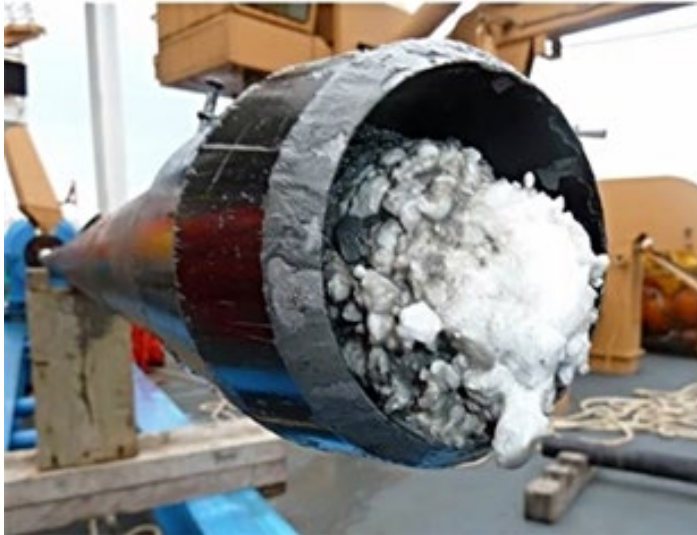
Figure 1: Hydrates Formed on a Pipeline.
