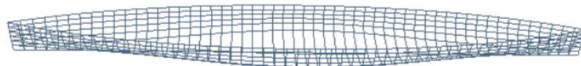
Figure 14: Total 648 panels is used to discretise Wigley form with 12 panels along the girth direction and 54 panels in longitudinal direction.
