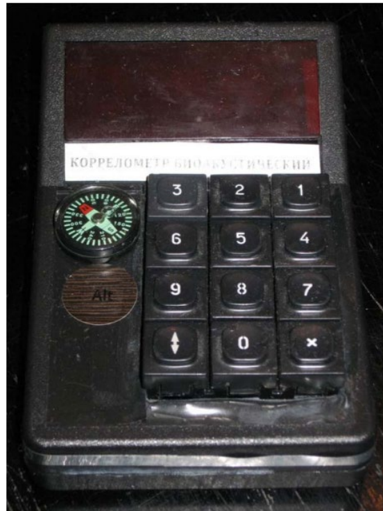
Figure 3: Digital microprocessor azimuthal bioacoustic correlometer for microphone arrays with ADCs. Prototype development: Adamovich E.D. (2015).
