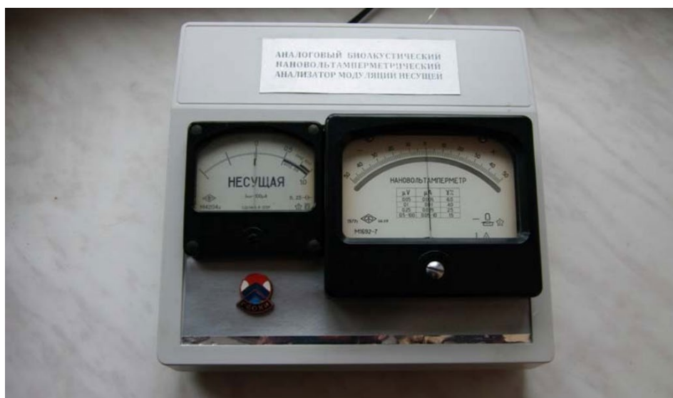
Figure 5: Precision digital bioacoustic carrier modulation analyzer with universal serial bus (USB) and built-in two-channel ADC. The left indicator is a carrier wave indicator. The right indicator is the low-inertia nanovoltmeter. This instrument was developed by Gradov O.V. (with co-authors) in GEOKHI RAS in 2010. This instrument was reconstructed and modernized by Adamovich E.D. in 2014.
