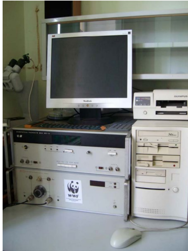
Figure 1: Computer-based modular analyzer of entropy, noise quality and phase with post-processing and analysis of bioacoustic signals in MATLAB, EDSW, "Fractan" and "AutoSignal" software (GEOKHI RAS, 2010).
