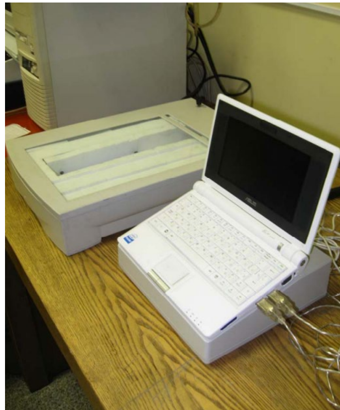
Figure 2: Elementary multimodal acoustochemical and bioacoustic (entomological) spectrometer with advanced spectral signal processing. General view of the device with a control panel and an ADC placement unit. The universal serial bus (USB) inputs leading from the ADC to the PC are visible (ICP RAS, Department of Dynamics of Chemical and Biological Processes, 2011). This device can also be used as a bioacoustic signal cepstrometer with ZLAB ADC-DAC.
