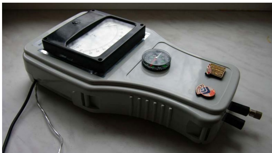
Figure 4: Multi-angle orientation comparative two-channel correlometer with a universal serial bus (USB) and built-in ADC. This instrument was developed by Gradov O.V. (with co-authors) in GEOKHI RAS in 2010. This instrument was reconstructed and modernized by Adamovich E.D. in 2014.
