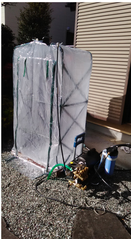
Figure 3: Photo of polytunnel equipped with mist former. The miniature polytunnel (69 x 49 x 124 cm), FGH 124, was purchased from CAINZ, and a set of mist former which was constructed with a nozzle and 0.8 LPM direct drive pump, #7527, was purchased from Green Com. Japan.
