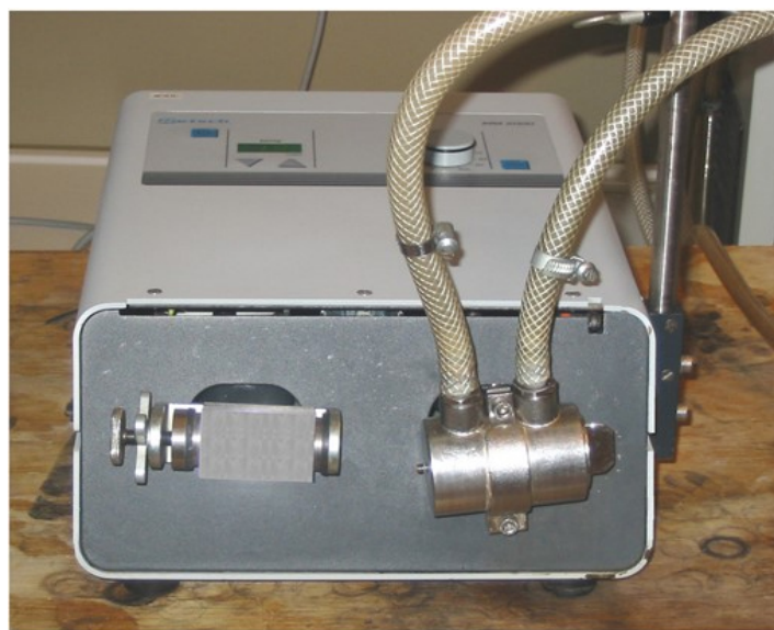
Figure 2: Lab-size shaker ball-mill MM200 ® from Retsch GmbH; the 20 ml beaker with temperature control proper milling times are minutes to at most 1h [5].
