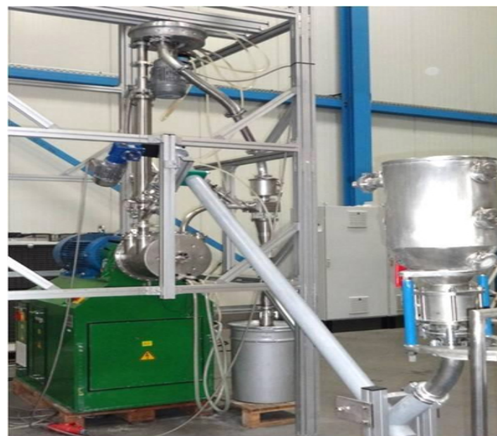
Figure 6: A 20 L Simoloyer ® at continuous operation; courtesy of Zoz Ltd. Wenden, Germany.
