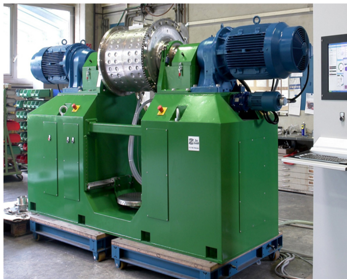
Figure 5: 100 L production unit horizontal rotor ball mill, set for inert gas operation courtesy of Zoz Ltd. Wenden, Germany [4].
