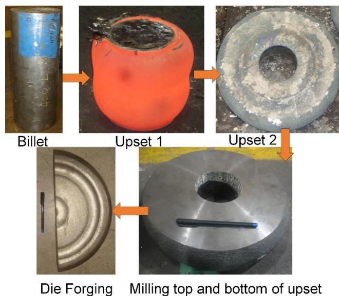
Figure 1: Forging process sequence finalized using simulation studies. Upset 1 and 2 carried out in hydraulic press and die forging carried out in pneumatic hammer [22].
