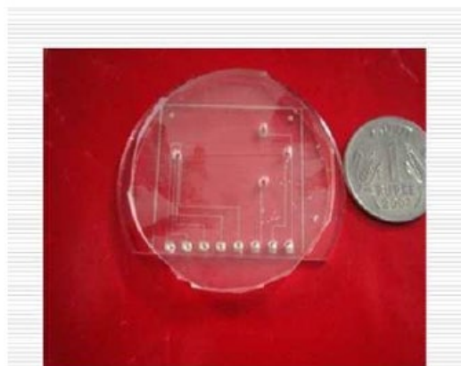
Figure 6: Complete Photograph of Integrated Lab-on-a-Chip Fabricated
