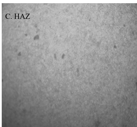
Figure 3: (C) Micrograph of OA Weld HAZ
