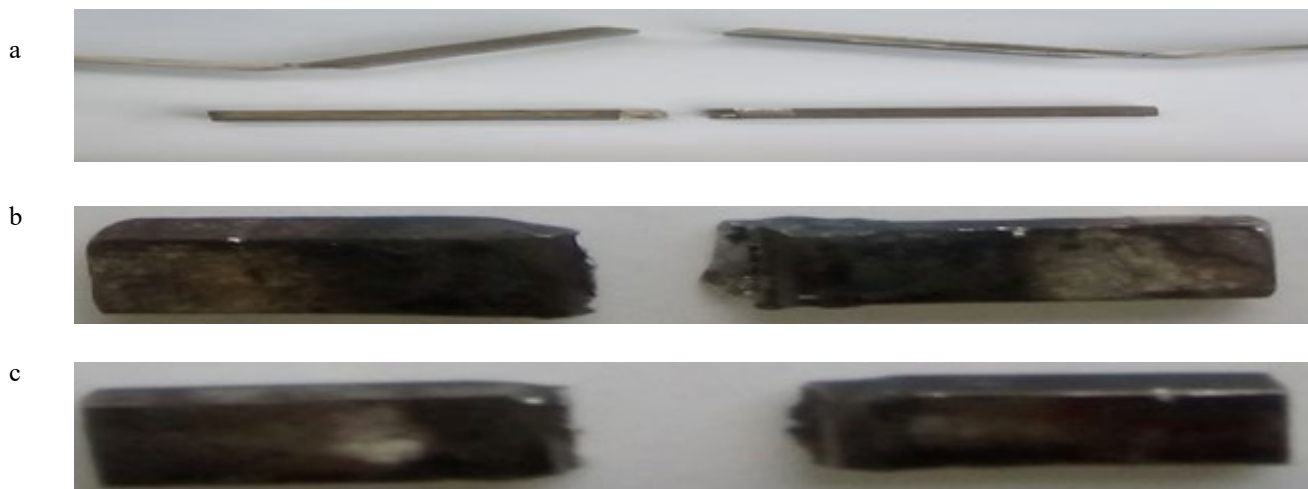
Figure 5: (a) Impact Behaviour of the Parent Metal, (b) Impact Behaviour of the TIG Welding, (c) Impact Behaviour of the OA Welding
