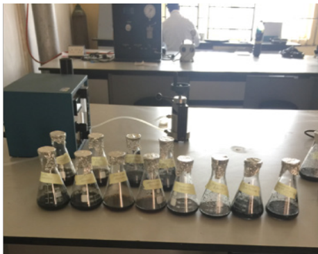
Figure 1.1: Produced water sample and filtrates from adsorption process
