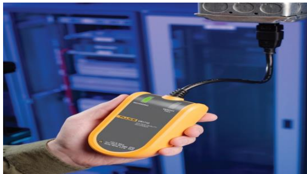
Plate I: Voltage Quality Recorder (VR1710) Sources: (a) Installation Manual of Fluke VR1710 (b) Power Outlet in Bauchi)
