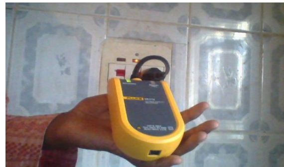
Plate I: Voltage Quality Recorder (VR1710) Sources: (a) Installation Manual of Fluke VR1710 (b) Power Outlet in Bauchi)
