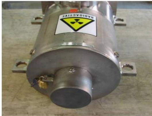
Figure 2: Illustrates the Shielding of the Radioactive Source Used
