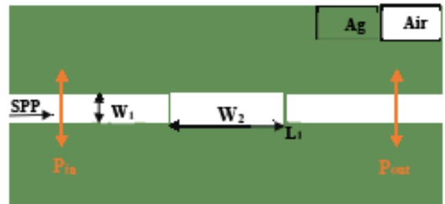
Two-dimensional Image of a Plasmonic Sensor with Two Waveguides and a Cavity
