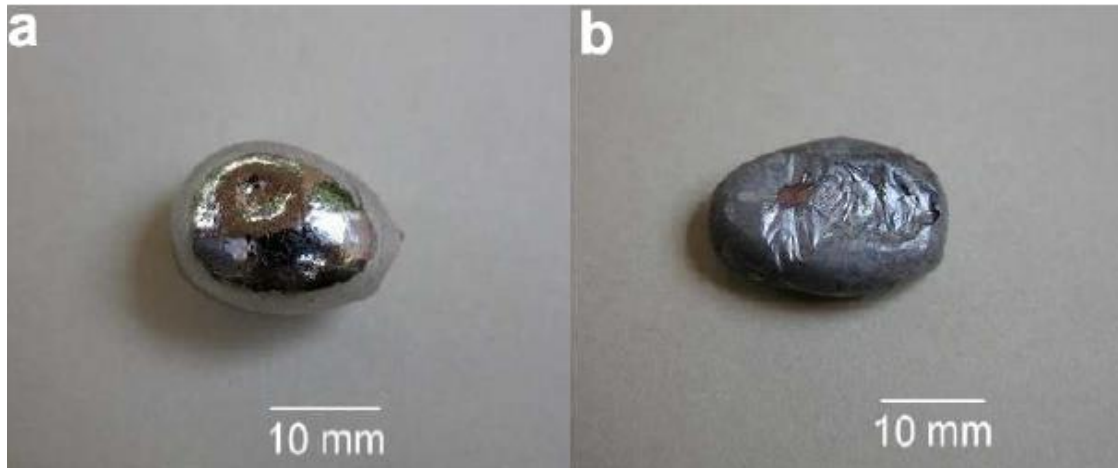
Figure 1: Samples Cuxwt%Nb-11-02 (a) and the sample Cuxwt%Nb-10-01 (b) immediately after they are melted in the arc furnace. If we look closely at the sample Cuxwt%Nb-11-02 (a) we perceive a typical brightness that is not characteristic of Cu (even this sample has x=80 % by weight of Cu). Microscopy images scanning revealed the migration of the Nb to the peripheral regions of the sample: " Cocoon Effect ".
