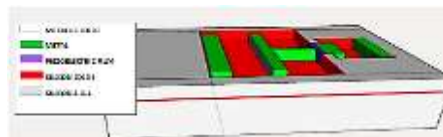
Figure 38: 12. Metal Deposit, Metal Engraving Etching of the Piezoelectric Layer
