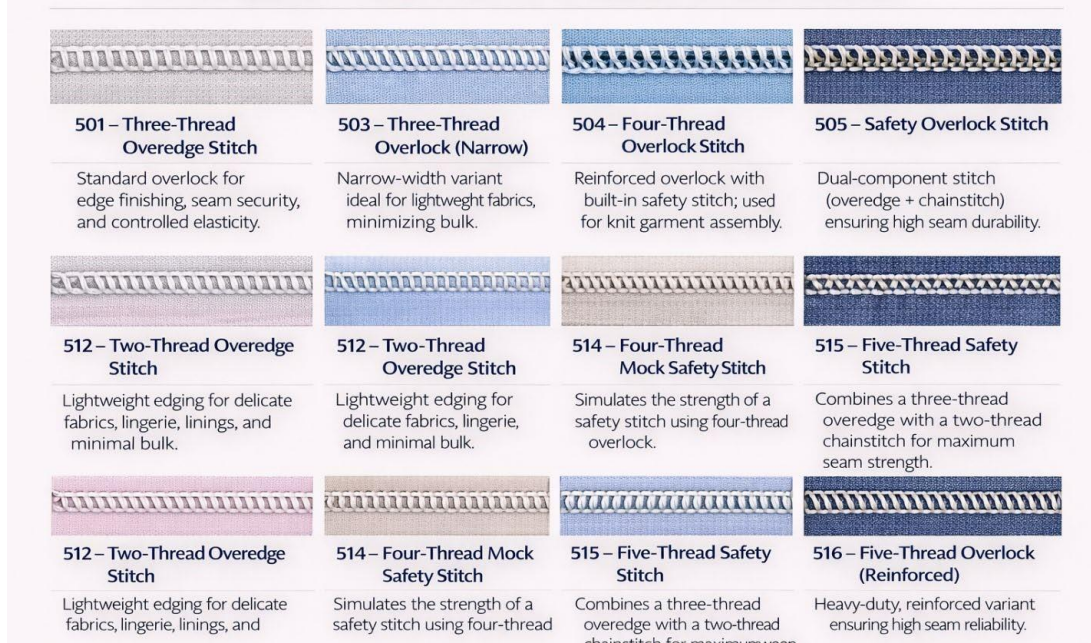
Figure 5: Stitch Types — Class 500 (Overedge / Overlock Variants) (ISO 4915 Classification)
