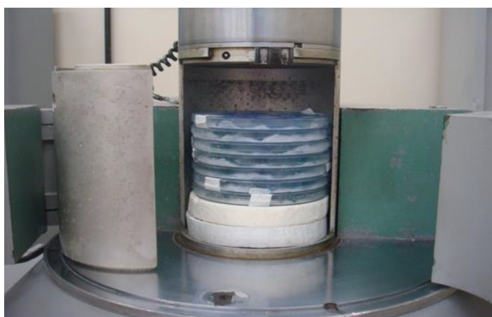
Figure 6: Placement of Petri's s plaques with different samples before submission to gamma irradiation.
