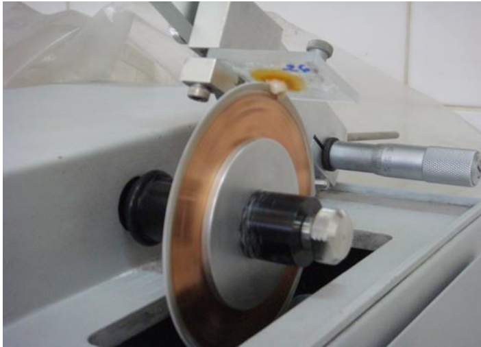
Figure 1: Cutting with fine-grained aluminum disc to obtain slabs from dental enamel.
