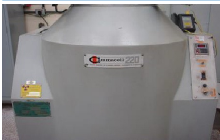
Figure 5: Cobalto-60 GammaCell irradiator source. Dose rate: 2 Gy / 4, 4 seconds, received twice daily (total dose: 72 Gy).
