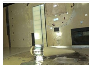
b) Mars exploration airplane wing and aileron controlled by a DE actuator in the 2mx2m low-speed wind tunnel experiment (JAXA: Japan Aerospace Exploration Agency).
