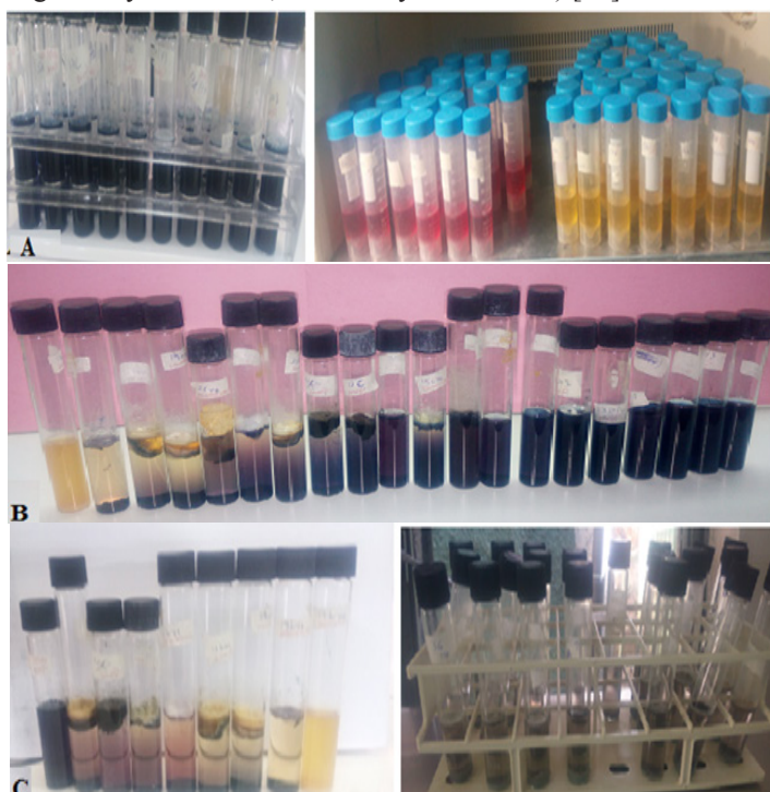
Figure 7: Azo dye degradation at the first day A:-Decolorization of Navy blue, Procion red MX-5B, Remazol yellow dye at the first day. B: - Decolorization of Navy blue, at 5 th day.C:- Decolorization of Navy blue, at the end of 9 th day
