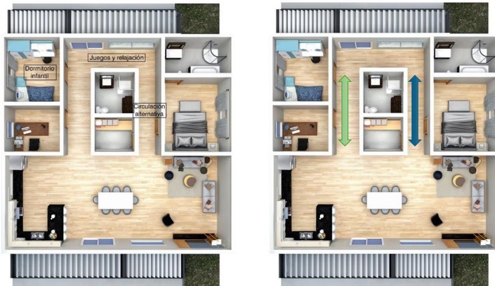
Figures 2.1 and 2.2: Alternative Routes with Activities Compatible with Circulation Areas. “Interweaving” Integrated into the Structure as a Moderating (Relaxation) interface in the Family area. Colored lines Indicate the Origin of the Corridors with Different Colors: Green and Blue in this case. Collaboration of Sofia Ossa Zuain. Architects.
