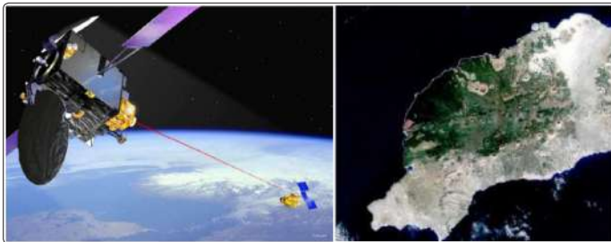
Figure 5 (a): Schematic depiction of SILEX inter-satellite link between SPOT-4 and ARTEMIS. (b). First image transmitted by the SILEX optical data-relay system, shows part of the island of Lanzarote, Canary Islands, and Spain [6].
