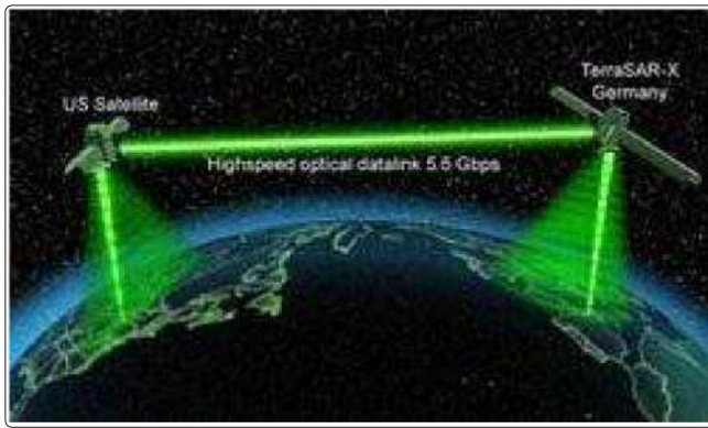
Figure 7: Intersatellite links between US Satellite and European Satellite using high speed laser [7]
