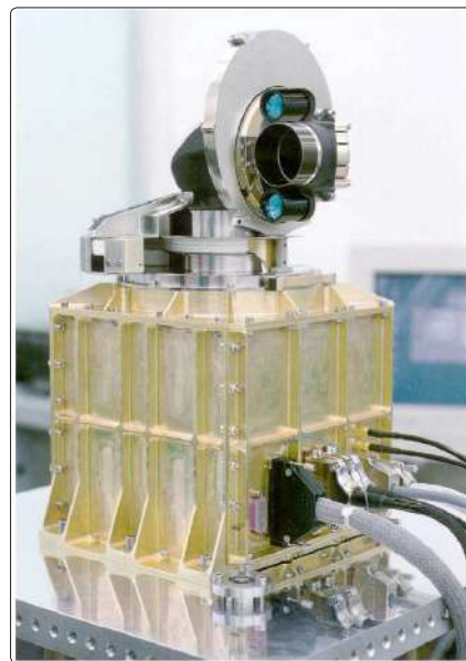
Figure 11: Engineering model of short range optical intersatellite links [13]
