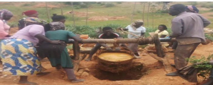
Figure 3: An image of locally extracted cassiterite using local hoisting mechanism at the study area
