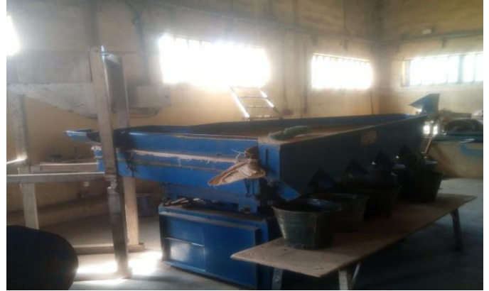
Figure 4: An image of Industrial Air float machine for processing the cassiterite using the action of vibration for even separation of the various minerals due to their different densities.
