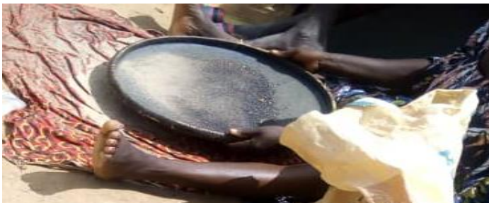
Figure 2: An image of semi processed cassiterite at the study area through the use of Panning Method
