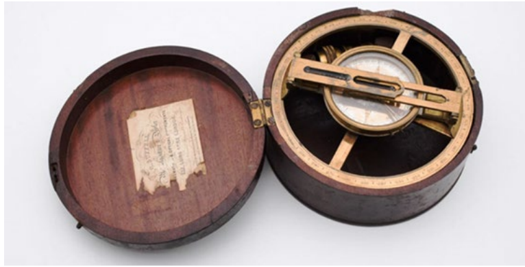
Figure 3: Troughton azimuth compass of the design Hochstetter may have used (00040567 National Maritime Museum)
