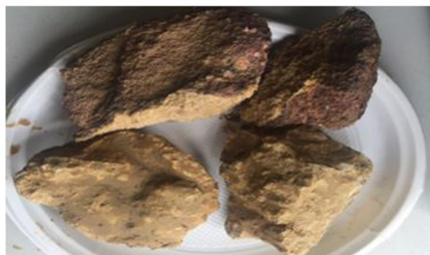
Figure 2: Sandstone samples after being immersed in drilling mud.
