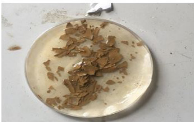
Figure 4: Mud cake sample during acidizing
