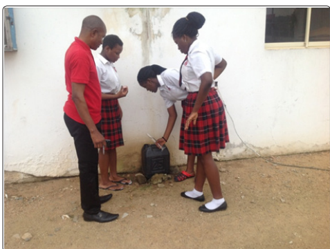
Figure 2.2.4: SDG team members pour 100 ml of diluted sulphuric acid into the digester under Mr. Salawu’s supervision
