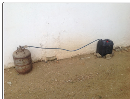
Figure 2.2.7: Digester is connected to the Gas cylinder by a tube on Friday, 26 th July 2019
