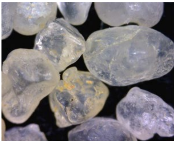
a: Sorted quartz gravel. Size: 0.8-1.5 mm
